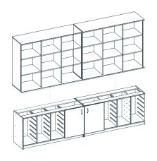
**Tip:** Fix Front of Class Unit Tops to wall prior to step 3.
