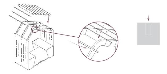
To position the roof, ensure the cut grooves are on the bottom and line up the corners with the stringer profile.
