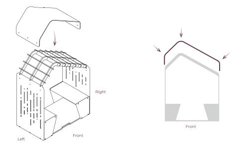
Push the fixing bars through the holes in the roof and sides. Fix in place using x6 20mm bolts.
